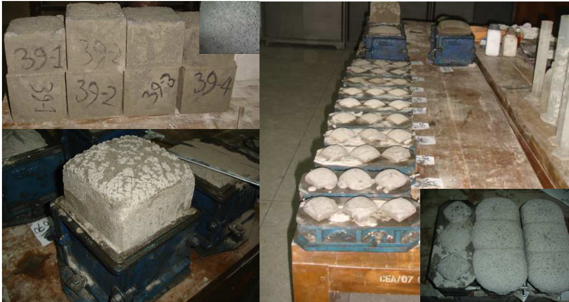
Figure 1: Volumetric expansion in cube sample and voids distribution in mortar matrix
